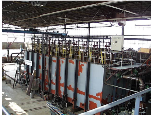
Figure 6. 1:4 scale hopper test rig “Schanulleke” at MTI Holland laboratories
