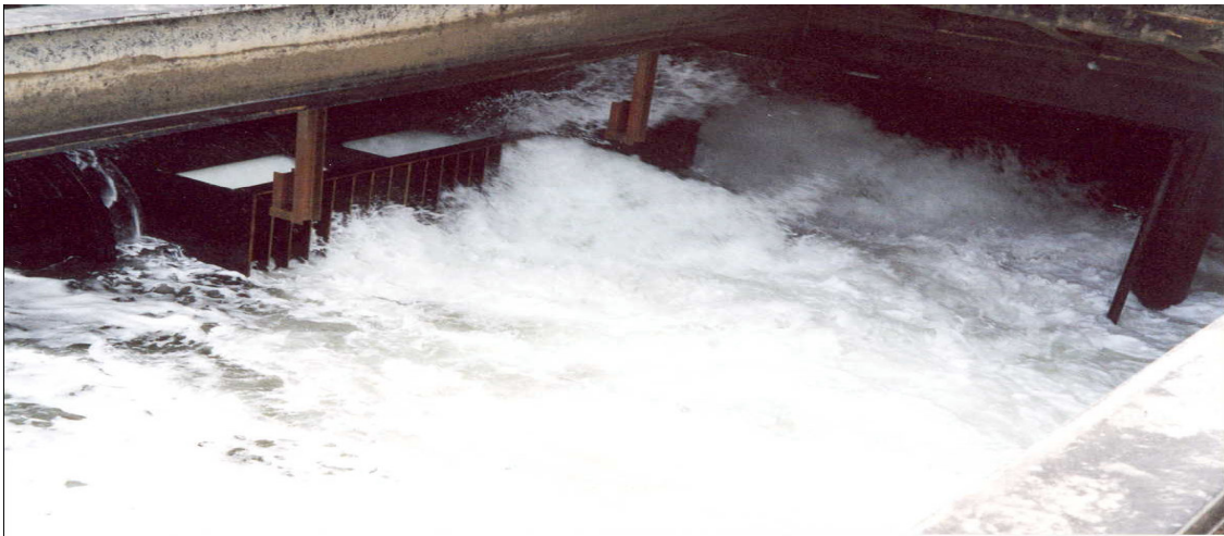
Figure 8. Full scale testing of Hopper loading box of new design
