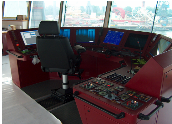
Figure 21. Single operator hopper dredger control desk (integrated dredging and navigation desk; first applied at TSHD Marieke)
