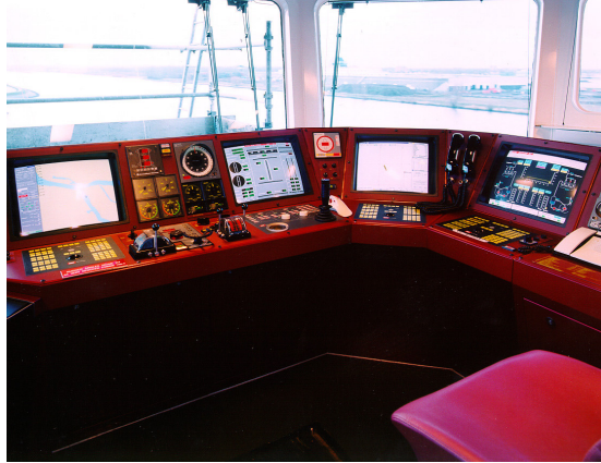
Figure 20. Integrated dredge automation; DP/DT, survey (DTPS), Radar, navigation and Conning
